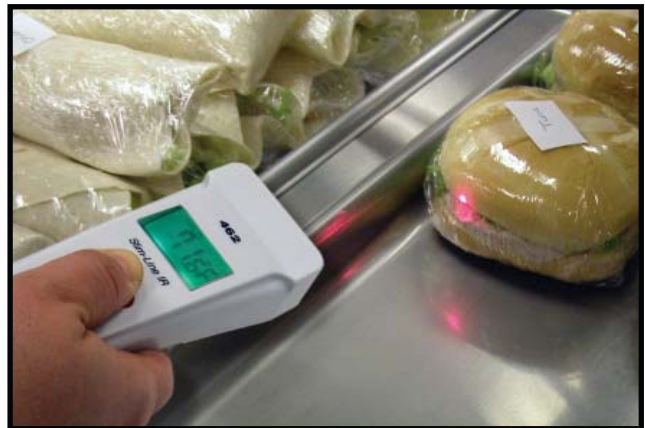
Non-contact means you avoid cross contamination of foods during HACCP temperature verification.
